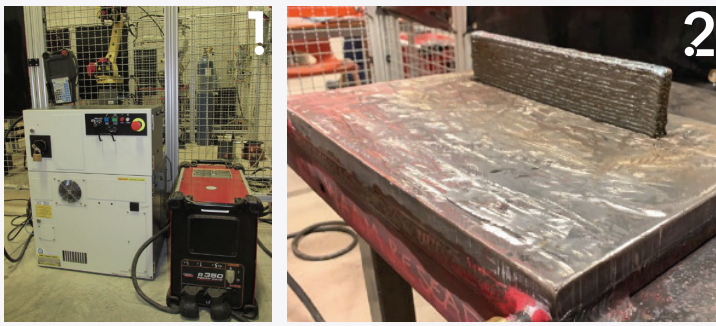
Fig. 1: Fanuc ArcMate 100-7L 6-axis Robotic Arm & Lincoln PowerWave R350 power source. Fig. 2: Water Cooled Steel Base Plate. Fig. 3: Experimental Weld Layers (length ~100 mm x ~16 mm wide). Fig. 4: Completed Tall and Wide Walls (300 x 100 x 16 mm) before removal from the base plate. Fig. 5: Typical Wall Straightness (less than ~2 mm per 300 mm height or width); Tall Wall shown on its side. Fig. 6: Close-up Views of a Typical Wall. Image 7: Welding Action Shot.
