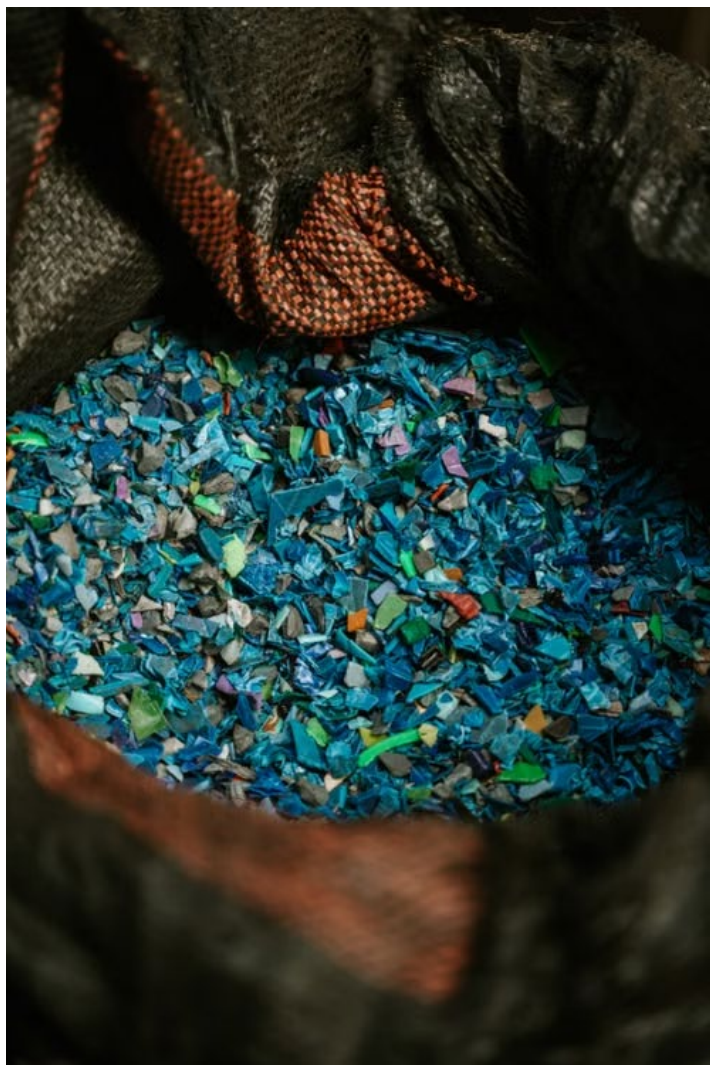
Figure 7. Processed post-consumer plastic prepared for use as recycled feedstock.
