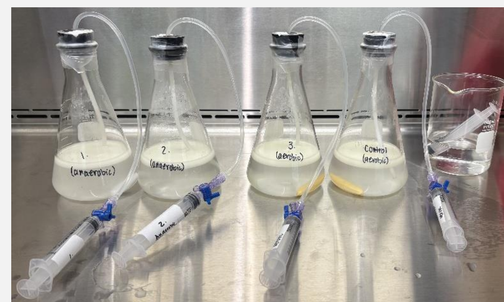
Figure 2. Luer lock system for flasks using 0.2" tubing, 3-port luer lock with adapter, rubber stopper with one hole and a sampling syringe.
