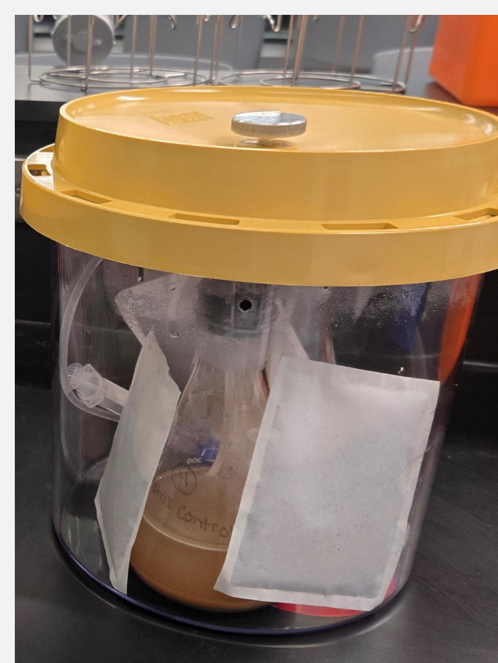
Figure 3. Flasks in airtight chamber under anaerobic conditions.
